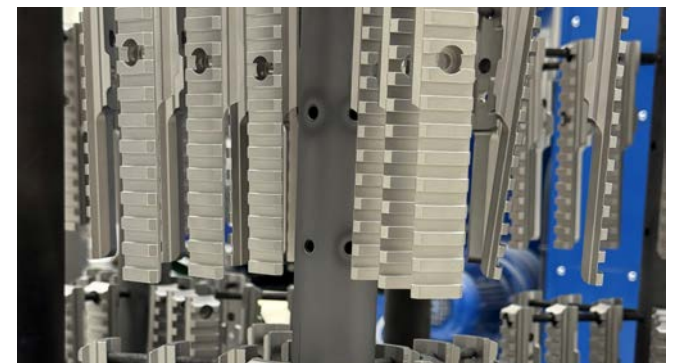
Riflescope mount for the MAUSER 25, ready for plasma oxidation.
